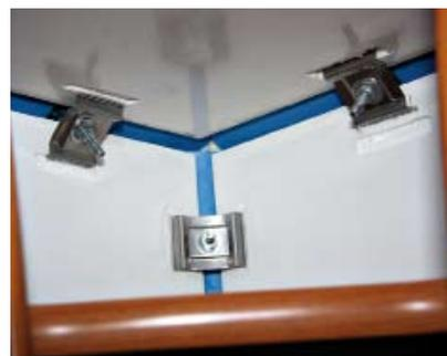
An early prototype showing the clamping system inside a roof locker
