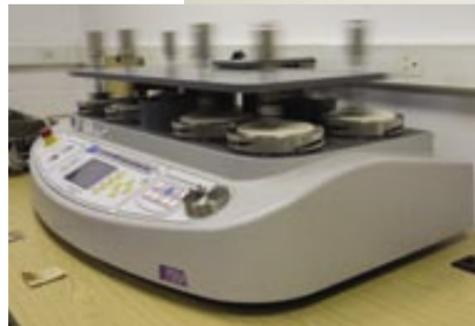
Oscillating pads are testing upholstery fabric for durability
