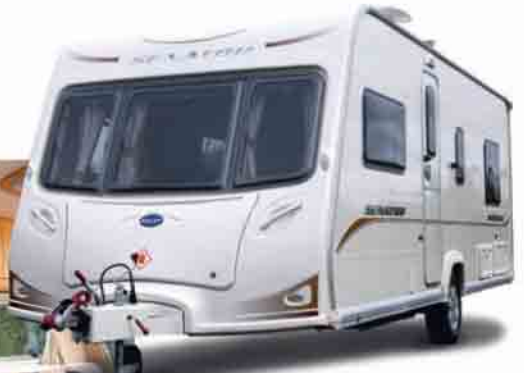
Stability aids include AL-KO's stabiliser and ATC systems
