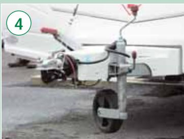
4. With the dummy towball in place and the cable tightened, its jockey wheel is held clear of the ground
