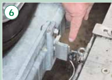
6. Each time the rotating caravan passes the mid-point, a switch keeps count and each cycle is timed
