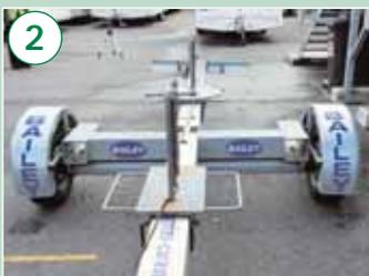
2. This trailer has weight-stacking points which can be positioned anywhere along the main central beam
