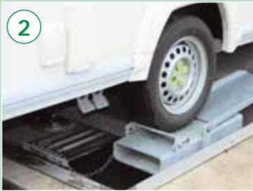
2. A caravan requiring evaluation is pushed along the ramps and chocked directly over the cross-beam
