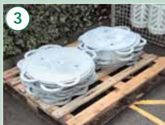
3. Steel weight plates can be mounted on the stacking points to create the loading mass required
