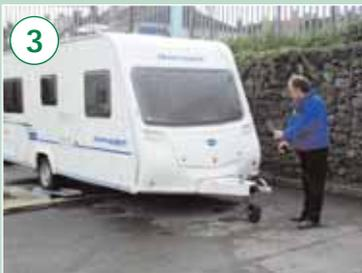
3. A dummy towball attached to an overhead cable is inserted into the caravan's coupling head
