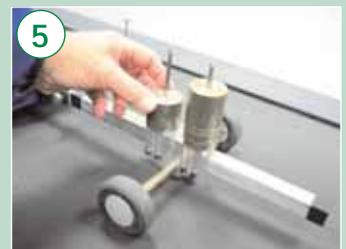
5. The rolling road is as authentic as possible and weights on the miniature trailer can also be adjusted
